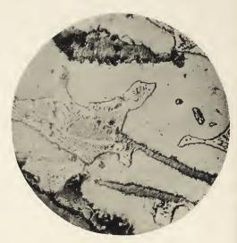
Fig. 24. Same as Fig. 26, but magnified 250 diameters. The compound character of the eutectic is very evident.
